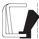
Ki Simple Labio sin Resorte Simple Lip without Spring
